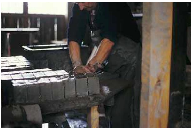
Making brick with traditional methods. Sweden. Photo Olof Antell.
